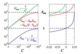
**Fig. S2.** System performance  $G_{max}$  (green),  $G_{min}$  (red), and  $S_{max}$  (blue) as a function of component values C for  $A_{min}$  = 100. Left has logarithmic units for C. In Right, note that, for positive feedback C > 0,  $S_{max} > 1$  and noise is amplified.
